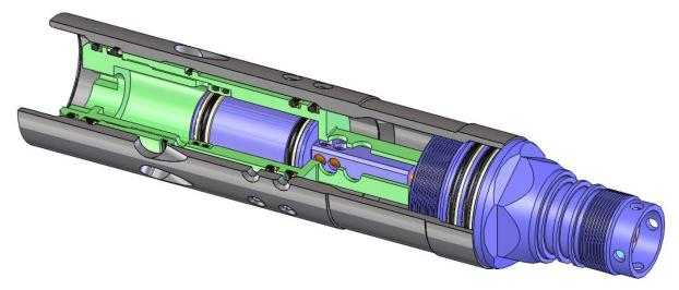
21. Use a socket wrench on the **Big Piston Top Cap** to align the **Piston Assembly** with the square cut out on the **Drive Sub**. The **Piston Assembly** will move past the flow ports on the **Main Sleeve** when it is fully inserted.
