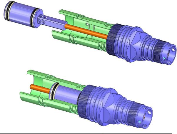
11. Remove the **Piston Assembly** from the **Drive Sub** by turning the **Coupling** counterclockwise. Gently press against the **Small Piston** while rotating the **Coupling** so that it remains fully inserted inside the **Big Piston**.
