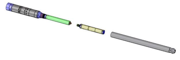
3. Remove the four **Socket Head Cap Screws** from the perimeter of the **Drive Sub** then remove the **Motor Assembly**. Keep the **Coupling** as it is required for future steps.
