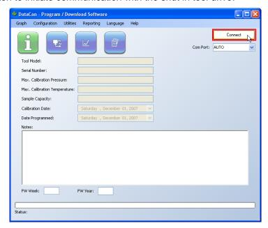
The **Tool Model**, **Serial Number**, **Valve Size**, **Housing Material** and **Sample Capacity** fields will fill with information.
