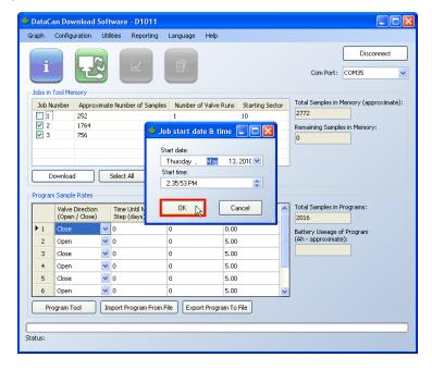
The software will now automatically convert the data file to a text (ASCII) file based on the settings (see Configuration section) saved in the tool memory. The status will read Complete when all of the selected jobs have been saved to the PC.
