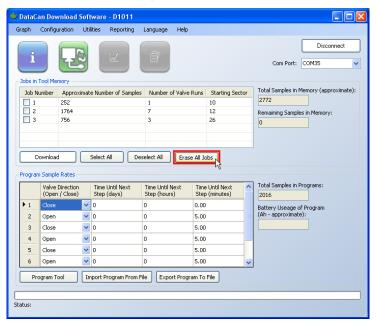
The status will read Complete when all of the selected jobs have been deleted from the tool memory. **Do not disconnect the tool or USB cable when erasing jobs from the tool.**
