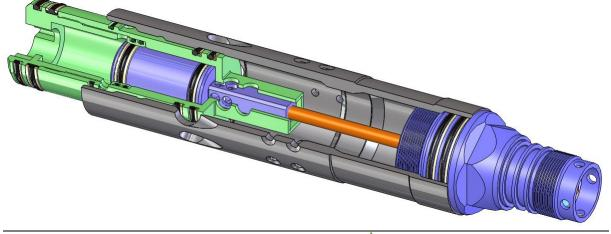
20. Thread the **Drive Screw** into the **Small Piston**. Turn the **Coupling** clockwise using a screw driver (or cordless drill) to pull the **Piston Assembly** into the **Main Sleeve**.
