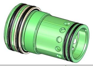
Install the first seal onto the **Big Piston** in the gland shown below. Use the **2-133 O-Ring**.
