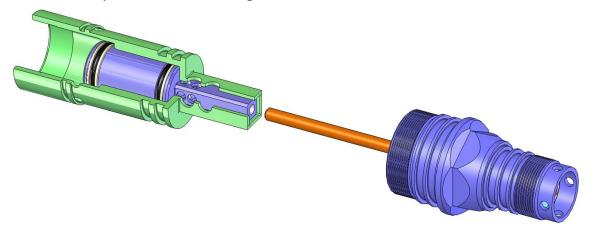
12. Install the LPT 224-2 T-Seal and TS-224 Back-Ups onto the Big Piston Top Cap. Apply o-ring grease liberally on the new seals.
