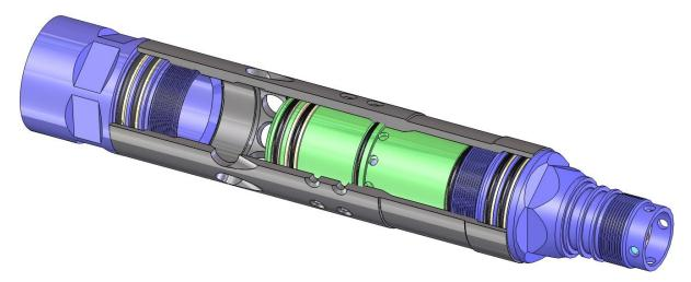
25. Install the **2-219 O-Rings** and **8-219 Back-Ups** onto the **Drive Sub** in the glands shown below. Apply o-ring grease liberally on the new seals.
