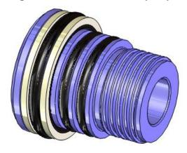
7. Install the **2-215 O-Ring** and the **8-215 Back-Up** onto the **Small Piston**. The back-up should be on the outside (closest to the square end).
