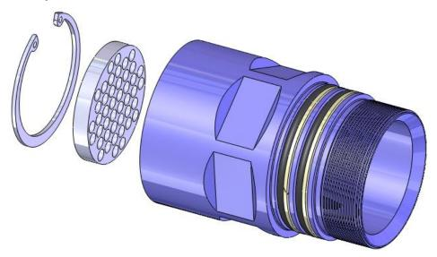
24. Thread the **Top Sleeve** into the **Main Sleeve**.
