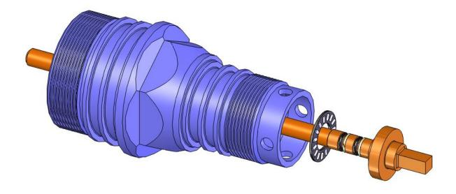
Install the second Thrust Bearing into the Drive Sub and place the Thrust Nut on top as shown below. Using needle nosed snap-ring pliers reinstall the Large Retaining Ring.
