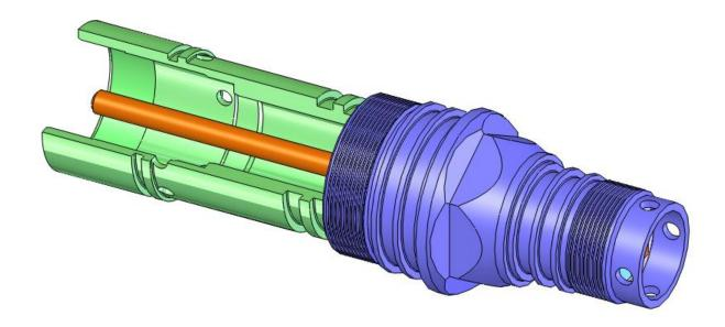
10. Thread the **Small Piston** onto the **Drive Screw**. Using the **Coupling** and a screwdriver (or cordless drill) turn the **Drive Screw** clockwise and pull the **Small Piston** into the **Big Piston**. To fully insert the **Small Piston** you'll have to align the male square end of the **Small Piston** with the internal square key of the **Big Piston**.
