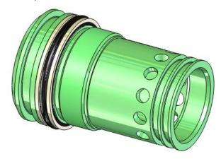
13. Install the remaining O-Ring seals onto the **Big Piston Top Cap**. The **2-127 O-Rings** go on the front glands, farthest from the T-Seal. The **2-224 O-Ring and 8-224 Back-Up** go on the back gland, next to the T-Seal.
