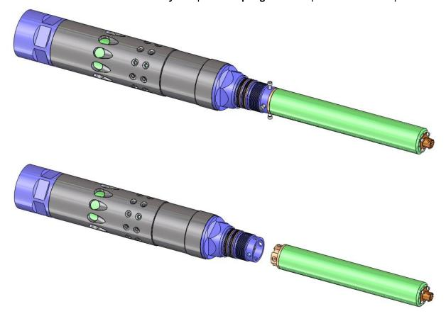
4. Place the **Main Sleeve** in a pipe vice, ensuring that the clamping point is away from the tool joints to avoid galling seal bores. Take care not to over tighten. Unscrew the **Top Sub** from the **Main Sleeve**.
