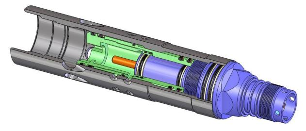
22. Install the seals on the **Top Sleeve** in the glands shown below. For the 2-1/2" Valve use the **2-226 O-Rings** and **8-226 Back-Ups**. Apply o-ring grease liberally on the new seals.
