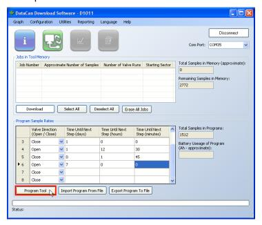
A pop up window will warn you that all jobs stored in the tool memory will be lost before the tool is programmed. If this is okay click the **Yes** button. **Do not disconnect the tool or USB cable when programming the tool.**
