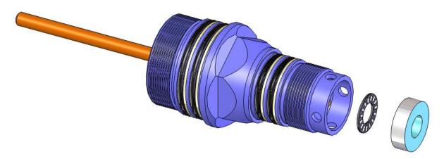
10. Push the Drive Screw and Thrust Bearing out of the Drive Sub.
