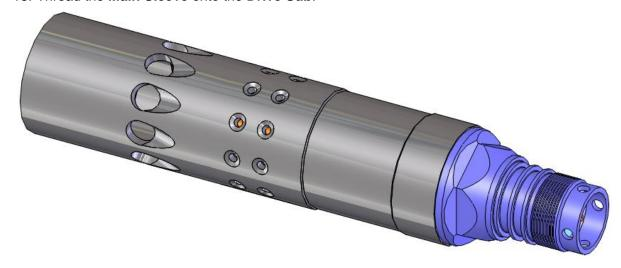
19. Insert the **Piston Assembly** into the **Main Sleeve**.
