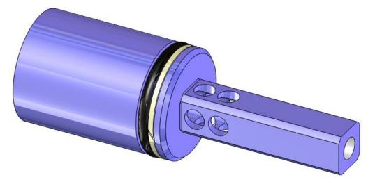
8. Thread the Small Piston Top Cap onto the Small Piston.
