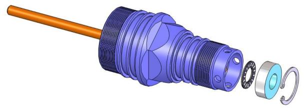
5. Install the LPT 215-2 T-Seal and the TS-215 Back-Ups onto the back gland of the Small Piston Top Cap.
