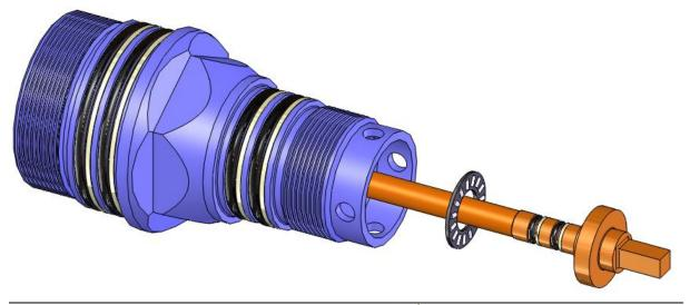
11. Push the **Piston Assembly** out the top of the **Main Sleeve**.
