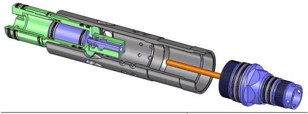
8. Using needle nosed snap-ring pliers remove the **Retaining Ring** from the **Drive Sub**.
