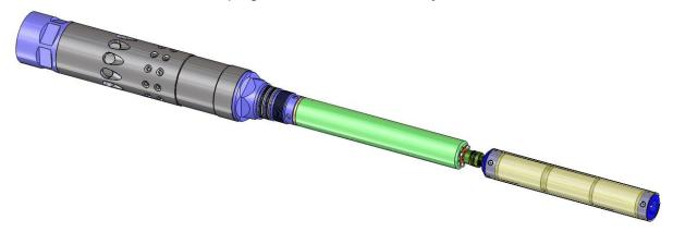
28. Thread the **Battery Housing** onto the tool. 30ft.lbs of torque is recommended which is similar to the force applied when holding the end of a 12" long wrench with two fingers.
