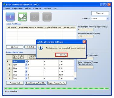
We recommend a surface test cycle at the beginning of every job. Program the valve for one open and close cycle at the surface before running the tool down hole.
