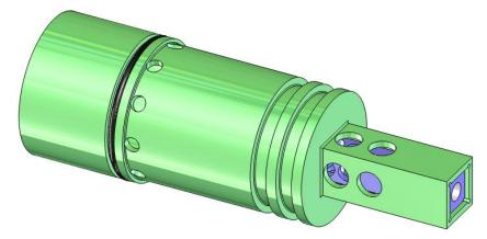
15. Install the second seal onto the **Big Piston.** Use the **2-223 O-Ring** and **8-223 Back-Up**. The Back-Up should be closest to the square end of the part. Apply o-ring grease liberally on the both of the new seals.
