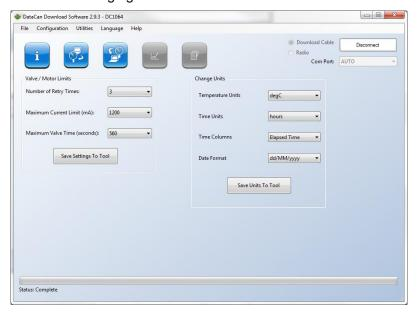
**Number of Retry Times**: indicates the number of times the valve will retry after a current setpoint has been reached. A retry will retract the valve for 5 seconds then reattempt the action. DataCan recommends 3 retry times.
