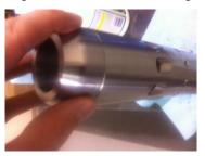
2. Push the housing into the test chamber with guide entering the chamber first.
