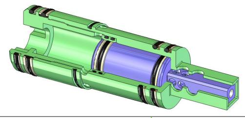
17. Install the **Drive Sub** seals in glands shown below. For the 2-1/2" Valve use the **2-226 O-Rings** and **8-226 Back-Ups**. Apply o-ring grease liberally on the new seals.
