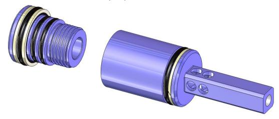
15. Using an o-ring pick remove all of the seals from the tool. Discard the used o-rings.
